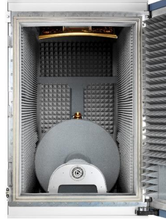
Figure 6: Rohde & Schwarz ATS1800C CATR system for UE conformance testing
