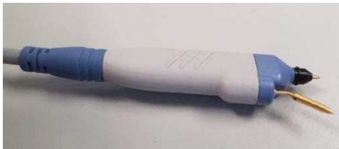
Figure 7 – R&S® RT-ZZ80 probe with the selected tips for the measurement
