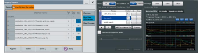
Figure 9: User defined frequency response correction on R&S@SMW200A and R&S@FSW
