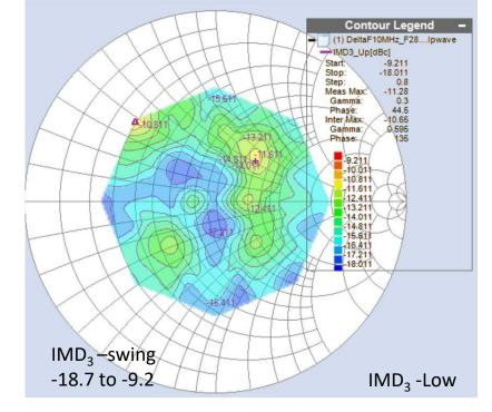
High Linearity achieved for both high and low side band at maximum  $\Gamma_{\text{OPT-Power}}$
