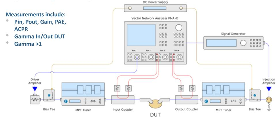
The tuning algorithm finds the optimum compromise for tuner loss and P<sub>ini</sub> for reaching Fload.
