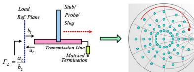
The movement of a stub/probe/slug in the horizontal direction alters the phase of the reflection factor
