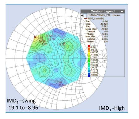
Fundamental load impedance fixed at optimum Pout Load impedance varied at 10MHz using LFT
