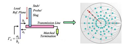
The movement of a stub/probe/slug in the vertical direction changes the magnitude of the reflection factor
