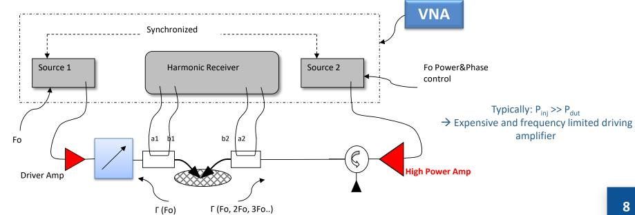
The disadvantages of this setup is that a very high power active loop amplifier is required to synthesize low impedance points.
